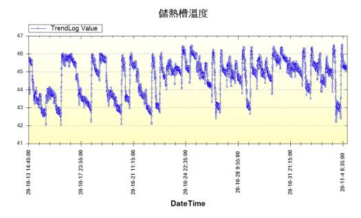
Over the past 3 weeks, hot water temperatures have been controlled between 42-46 C. The demand for hot water increases due to the colded weather; as a result, we have checked every setting of related equipment to cope with students' needs. If you have further questions, please do not hestitate to contact your dormitory supervisor or Chengkung Administration and Energy Management Section (Please contact extension number 3678 or fill out E-Form No. 1628.). 住宿服務組回覆:
